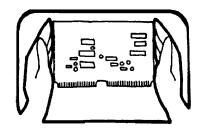
When removing plug-in assemblies, handle only by non-conductive edges and never touch open edge connector except at static-free work station. Placing shorting strips on edge connector usually provides complete protection to installed devices.
